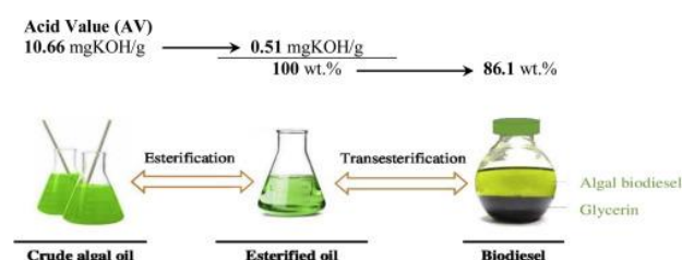
Figure: 2 Lowest AV with max. esterified oil yield (43%) at 12:1, 1% H 2 SO 4 , 60°C and 400 rpm for 90 min. Max. yield of biodiesel (86.1%) at 9:1, 65°C, 0.75% KOH, and 600 rpm.
